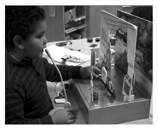
There are two types of actors – readymade actors for the prewritten piece, and recorder actors tho which new lines can be recorded by the players. The stage bow also contains a loudspeaker. The prewritten piece is presented in a booklet that explains the moves of the characters on the stage.
