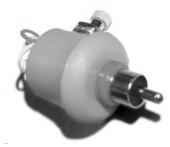
The contacts at the bottom of each actor: an audio plug connected to an ID tag, and a pushbutton to record or play back a recorded phrase.
