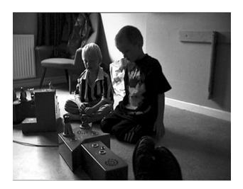
The physical set-up of the AudioTheatre consists of a "stage" with twelve contacts, and a number of painted backdrops. The "actors" are paper dolls cut in foam, placed on a plastic plugs with a small switch. Both paper dolls and backdrops have ID tags that can be read by the computer. The stage box contains a loudspeaker.
